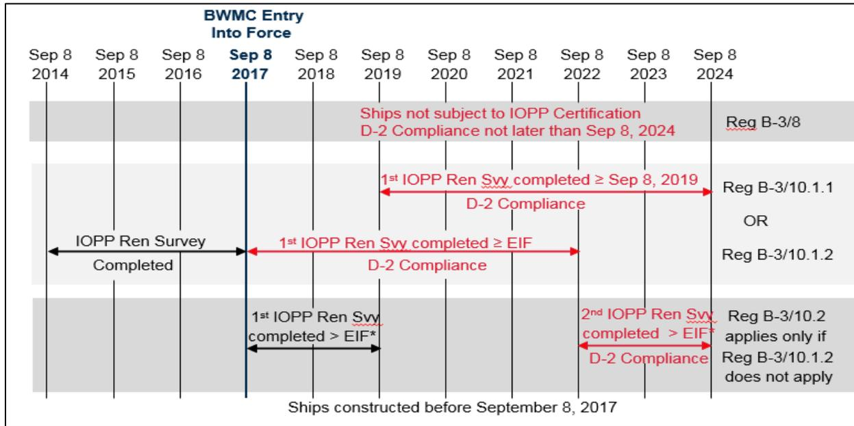
The amendments to regulation B-3 of the BWM Convention, which enters into force on October 13, 2019, requires ships constructed on or after 8<sup>th</sup> September 2017 to comply with the D-2 biological standard upon delivery. Referring to above diagram, ships constructed before 8<sup>th</sup> September 2017 are to comply with the D-2 standard at their **first** MARPOL IOPP Renewal Survey completed on or after:
